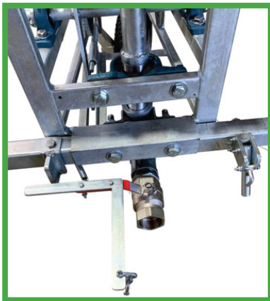
Pic 1: General arrangement, valve is in the shut position.
