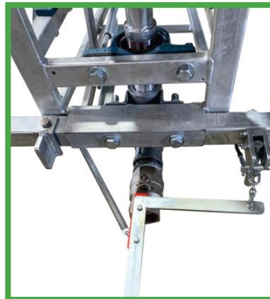
Pic 5: Shows mechanism 'loaded'. Valve is in the open position.
