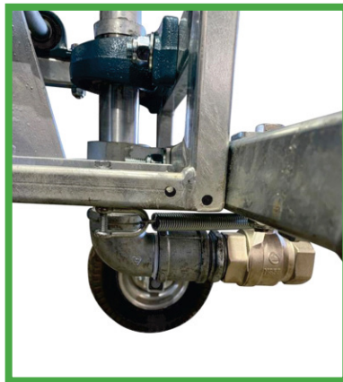
Pic 2: Connection of spring to the frame. D shackle is screwed on to an M6 bolt.
